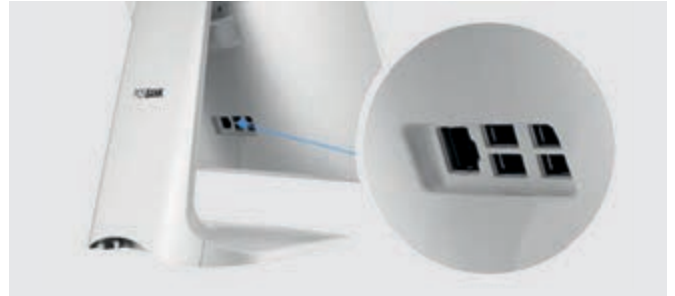
Multiple I/O interfaces • 6 USB ports, 6 Serial ports, and more
