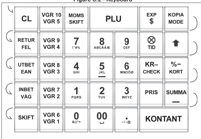
Figure 8.3 - Optional programmable keyboard
