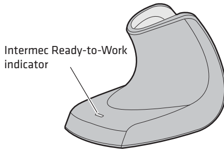
SG20 Bluetooth Base Station Ready-to-Work Light
